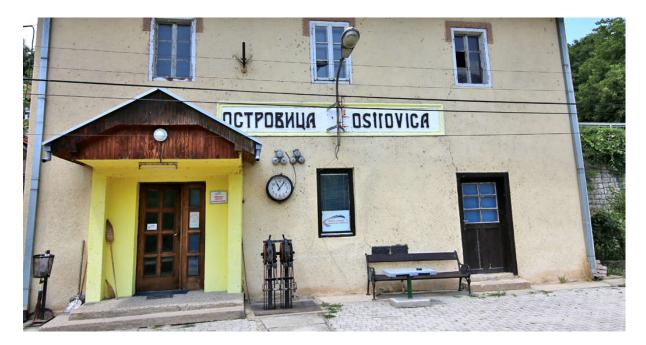
Figure 7. Ostrovica railway station, July 16, 2020 (Photo: Z. Cvetković) The station name, announcement bells, official clock, winches for remote lowering of barriers at the protected level crossings
