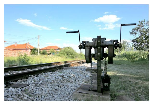
Figure 10. Winches for remote lowering and liftingbarriers at the level crossings in Srećkovac, July 15, 2020 (Photo: Z. Cvetković)
